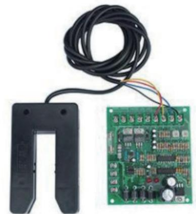
High precision photoelectric edge detector with the controllable distance being 2-5mm
